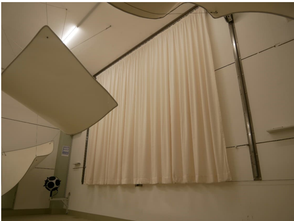
Figure B.2. Pleated hanging curtain in the reverberation room (diagonal view).
